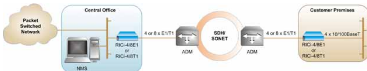
Figure 2. RICI-4E1/T1, RICI-8E1/T1 Extends Ethernet Services over Multiple E1/T1 Circuits
