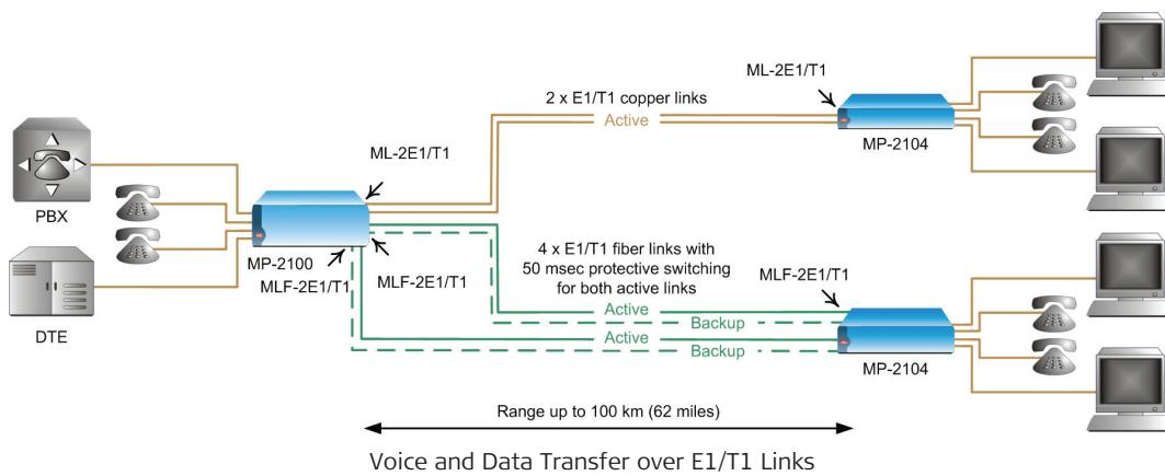
Additional main link modules can be installed in the Megaplex-2100 chassis to operate as hot standby modules. The backup module's links and the active module's links are connected to the same E1/T1 lines via Y-cables, providing full redundancy in case of main link hardware failure. Alternatively, multiple links can be configured for load sharing with optional priority bumping, ensuring continuous operation of the most important channels if one of the links fails.
