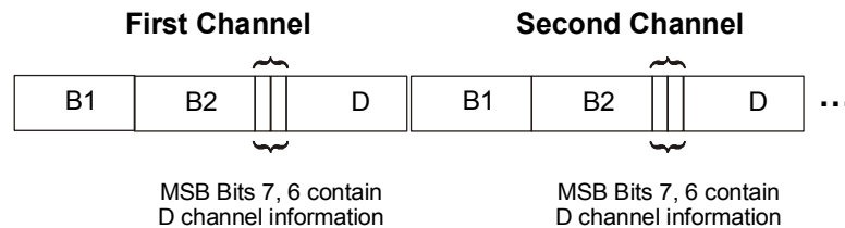
Figure 1-10. Timeslot Assignment in a Bundle, for IPmux-1E/ISDN
