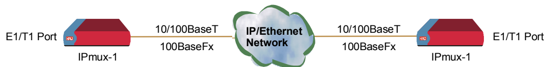
Figure 1-8. IPmux-1 E1/T1 Point-to-Point Application
