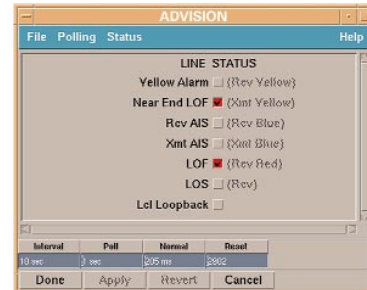
DS1 Line Status. Through a series of status screens the current device status can be displayed for pinpointing network problems.
