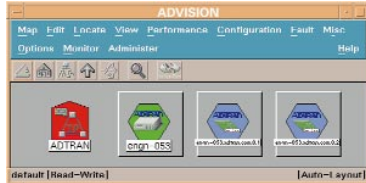
The OpenView submap for the DSU IV ESP. When HP OpenView discovers an ADTRAN SNMP device, ADVISION populates the submap with executable symbols for status reporting and GUI launching.
